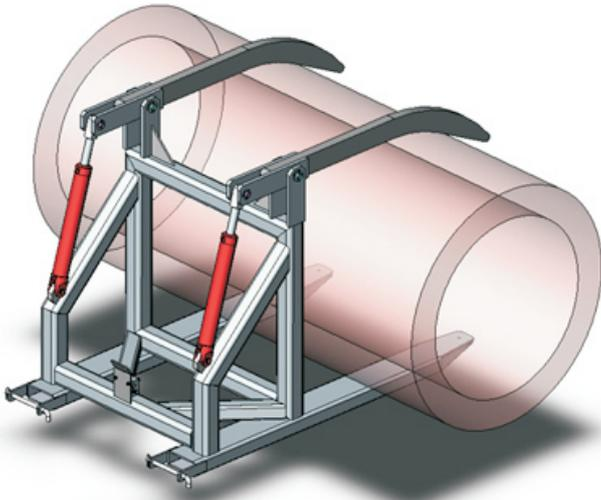
The type NS-GA-12 Grab Attachment has been designed to grab and secure poles or pipes from 300mm to 1200mm in outside diameter and safely lift and transport these by Forklift about the worksite. This slip-on attachment can be fitted in seconds to a forklift requiring only the connection to the 3rd function hydraulics, via the quick connect hydraulic couplings, and the installation of two locking pins supplied to prevent the unit from moving off the fork arms.
